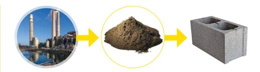
Fly ash is used to make cement and other concrete products.
